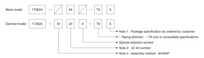
**Note1)** In taping packaging of products groups according to the  $\Delta C$  classification, products must be divided according to the group. If taping is performed without grouping into categories, products from two different groups may be mounted on the same tuner, so that  $\Delta C$  cannot be assured during tuning, making tuning defective.
